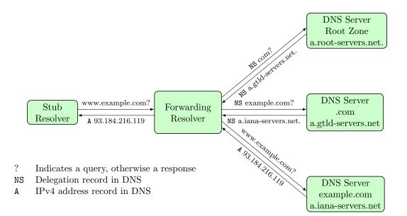
Figure 8: With query minimization, resolving the name www.example.com no longer exposes the full name and query type to the root zone and the .com authority. Naturally, this scheme still leaks quite a bit of sensitive information to the TLD's DNS server. Furthermore, the effect is even weaker in practice, as root zone is already often not contacted as information about TLD name servers is typically cached at forwarding resolvers.
