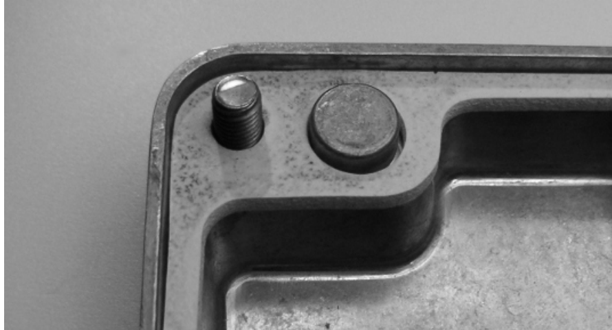
Figure 5.1.: Upper part of the aluminium containment with 3 mm thick silicone rubber sponge seal.
